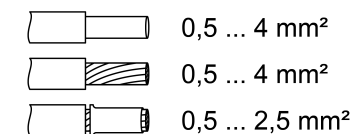
Figure 5: Clampable conductor cross-section
