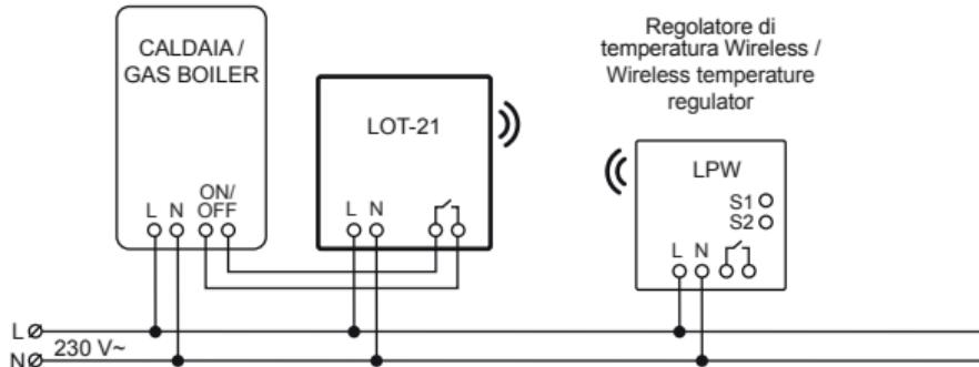
**EN** LOT-21 is a radio receiver for a controller (boiler) supplied with 230 V~. The main task of the device is to cooperate with radio temperature controllers or radio underfloor heating strips LLM-21. The receiver intelligently analyses states from controllers or strips and controls the switching on/off of the heat source (boiler, heating mat, heat pump). With this solution, a wireless connection between the controllers or slats and the heating source is possible.
